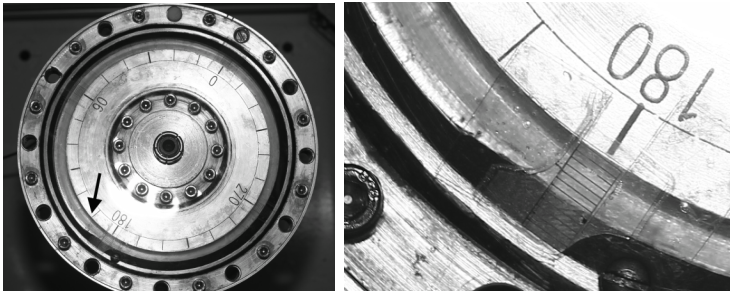
Figure 3: Hydraulic jump on the liquid layer in a cylindrical cavity with the rotational velocity satisfying the resonance condition \Omega = 1.25 \Omega_0 = 10 \text{ Hz}
