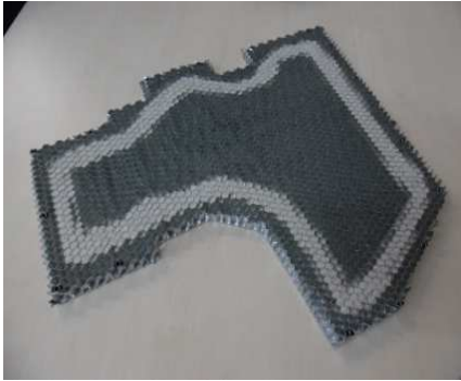
Fig. 8: Honeycomb bottom with sand filling at the border area.
