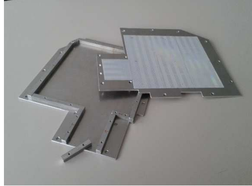
Fig. 3: Design of the oil pan bottom prototype I, with one large cavity for granular material.
