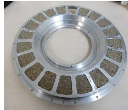
Fig. 6: Open part of the housing of an electric engine fully filled with granular material in large cavities [7].
